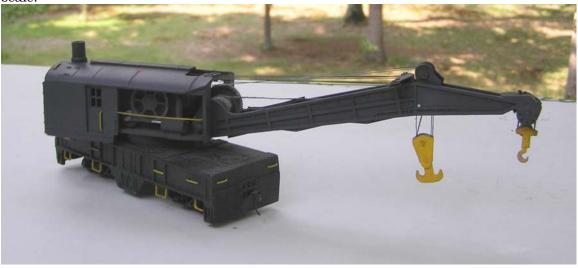
The derrick is a bash of a Lionel crane which scaled out as an S scale 200 ton Bucyrus crane. I chopped it down in length to be match that of a 150 ton crane, opened up the side, added gears and pulleys(from various bottle caps), added the reeving (cabling that lifts the crane and hooks) and scratch built the hooks. It is modeled after the Lehigh and New England's crane #700. (It took second place in the Maintenance of Way category at the SER contest.)
